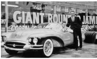
The lead image and the photo above shot at Skinner Buick in an unknown location feature the 1954 Buick Wildcat II Motorama concept car constructed by the Buick Division of General Motors. This unique show car was constructed on a Corvette chassis equipped with a supercharged Buick V-8. The Wildcat II fiberglass body shared the cutaway front fender styling cue with the 1954 Buick Skylark and utilized a one-piece Wildcat II hood and fenders with the headlights mounted on the bumper.
